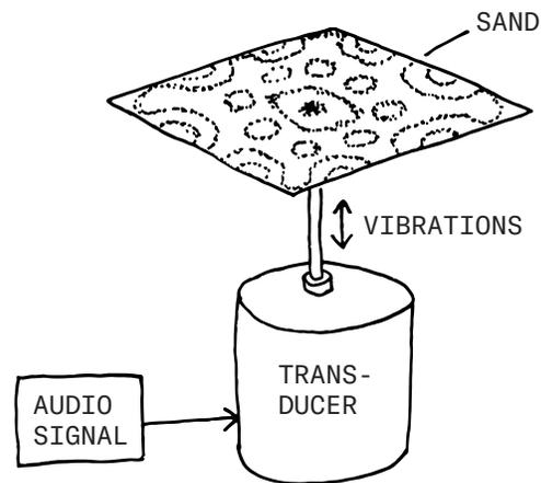
**Figure 25.** A Chladni plate driven by an electromagnetic transducer. The original version, invented by physicist & musician Ernst Chladni in the 1700s, used a violin bow to vibrate the plate.
