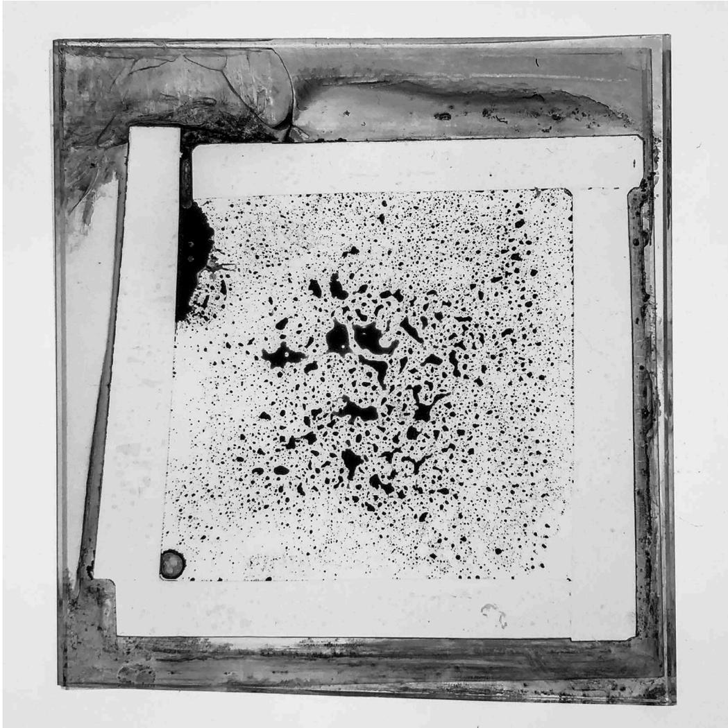
**Figure 32.** *Ferrofluid cell attempt #1: proof of concept. Glass spacers and UV glue. This was constructed all in one day, whereas the rest were built as a batch over the course of months. The ferrofluid stuck to the glass quite badly, but I was able to use it for testing of my magnets, shooting rig, and macro lens.*
