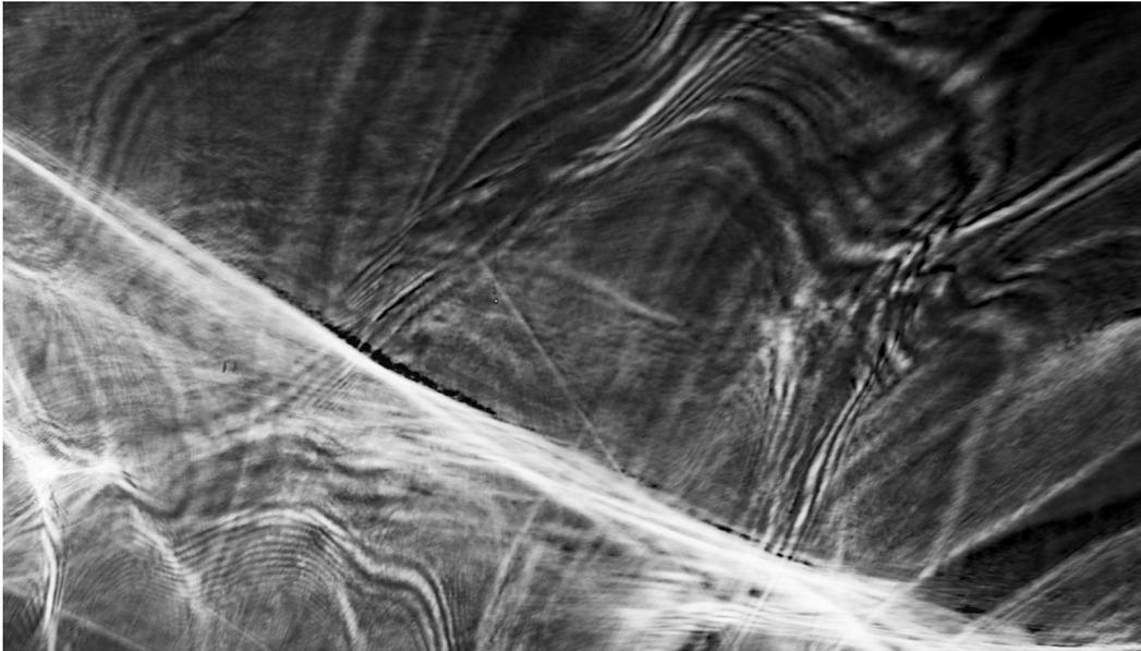
**Figure 17a.** Channel 1 of Refraction/Projection: stop-motion recording of refracted light from rotating glass object, captured by image sensor with no lens
