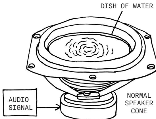
**Figure 26.** A speaker cone being used as a transducer for liquid cymatics.
