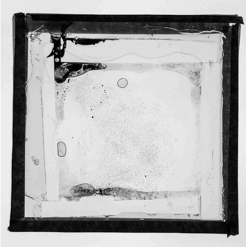
**Figure 35.** *Ferrofluid cell attempt #4. Glass spacers and UV glue, with additional silicone sealant applied around the outside edges. This cell was reasonably successful, and I used it to shoot my "rehearsals" of the final piece. The ferrofluid left behind a trail of very small dots, but it had the least sticking of any cell.*
