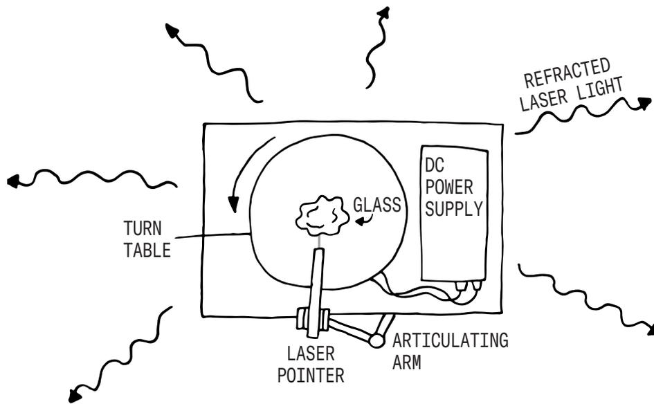
*Figure 14. The apparatus for Lumiagraph*
