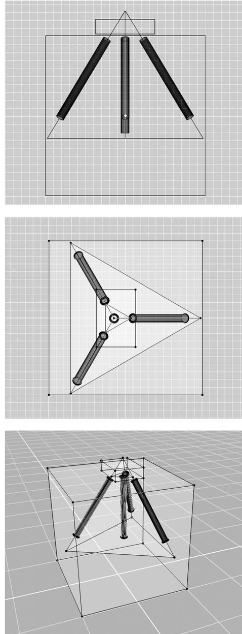
**Figure 45.** The four electromagnetic coils are shown relative to the cube from the side, top, and perspective views. I had trouble illustrating the geometry of the coil placement using pen and paper, so I modeled them in 3D using Blender.
