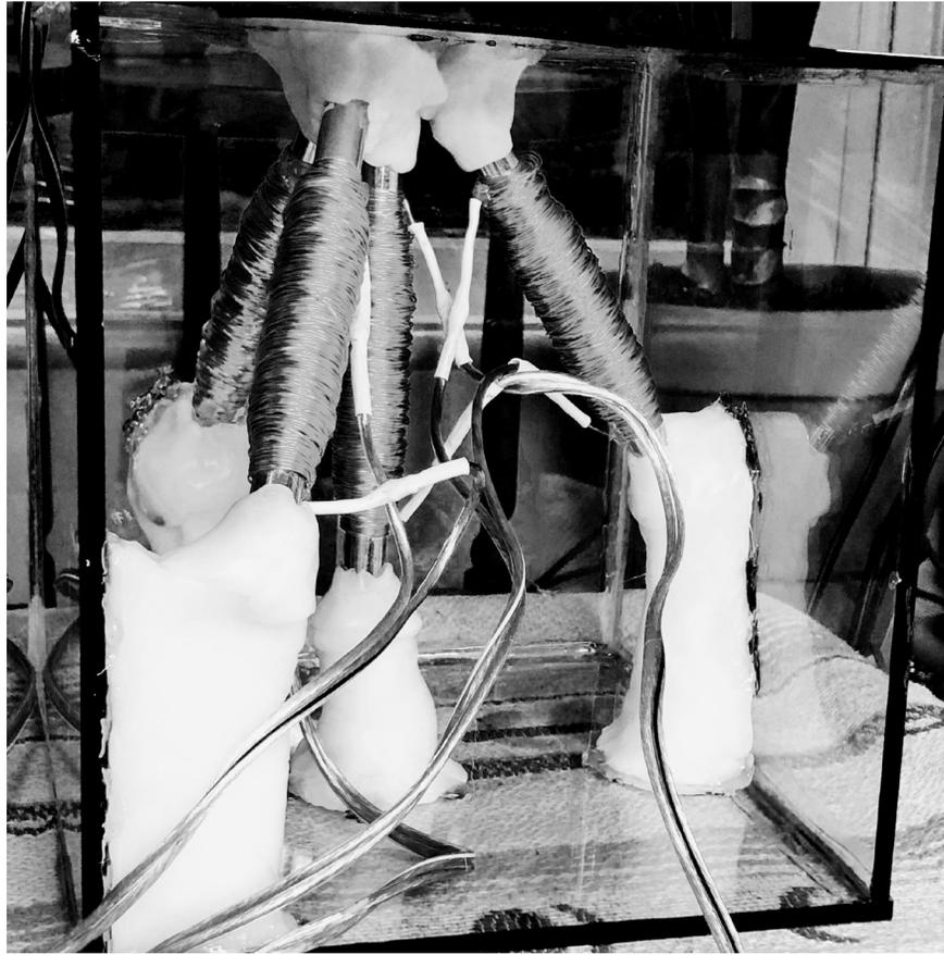
*Figure 43. The electromagnetic coils mounted inside the glass cube.*
