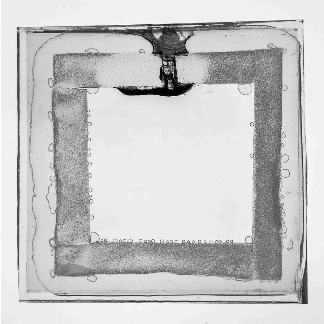
**Figure 33.** *Ferrofluid cell attempt #2. Weather tape spacers and silicone sealant. This cell did not have a good seal, so it dried out completely and was unusable.*
