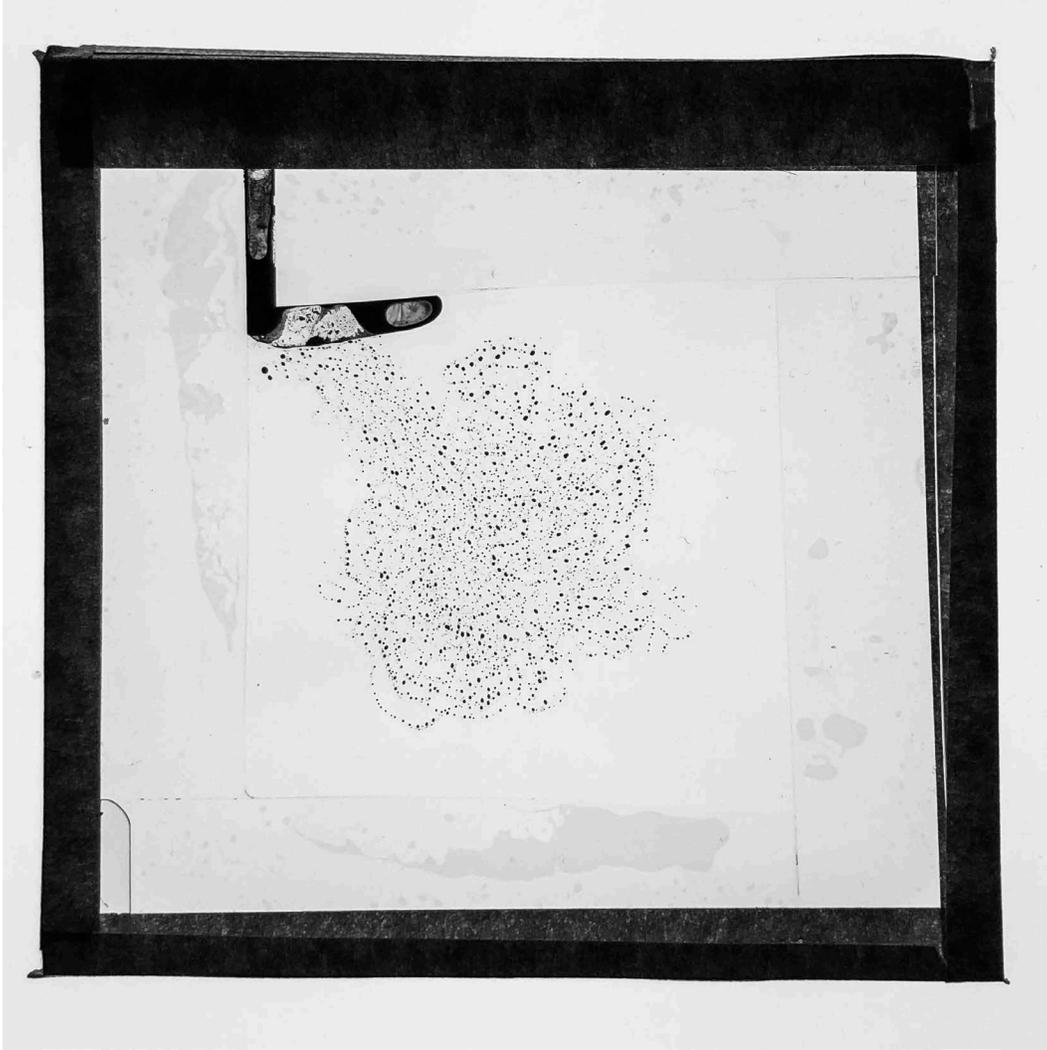
**Figure 36.** *Ferrofluid cell attempt #5. Glass spacers and UV glue. This cell was the most effective of the batch, with very little staining and air bubbles. The trail left behind from the ferrofluid consisted of larger dots than attempt #4, but it did not interfere too much with my shooting. This cell was used to shoot the final recording for Labyrinthine.*
