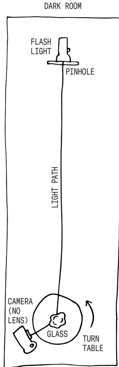
*Figure 18. Shooting setup for channel 1 of Refraction/Projection*
