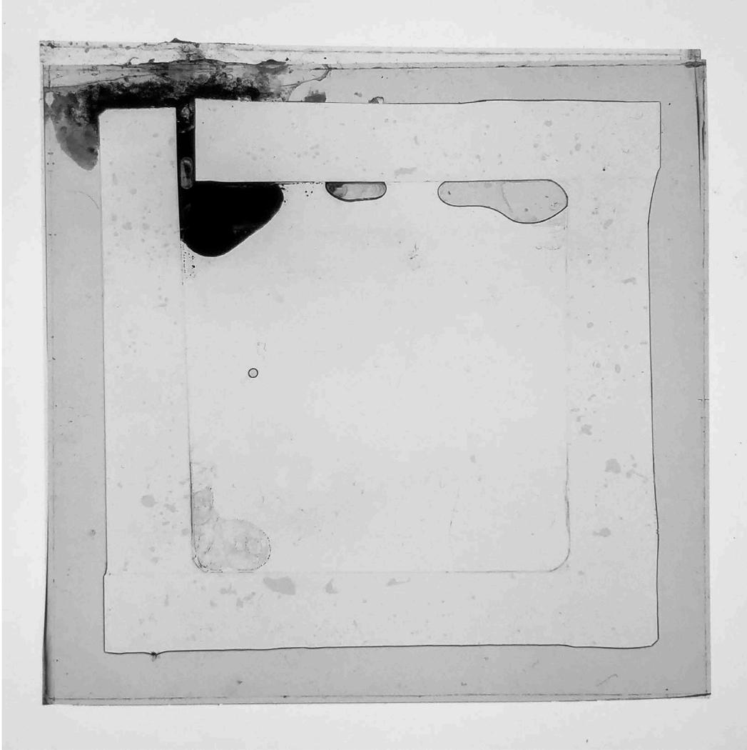
**Figure 34.** *Ferrofluid cell attempt #3. Glass spacers and UV glue. This cell had a good seal, however there was some debris and pockets of air that found their way inside which would have interfered with shooting.*
