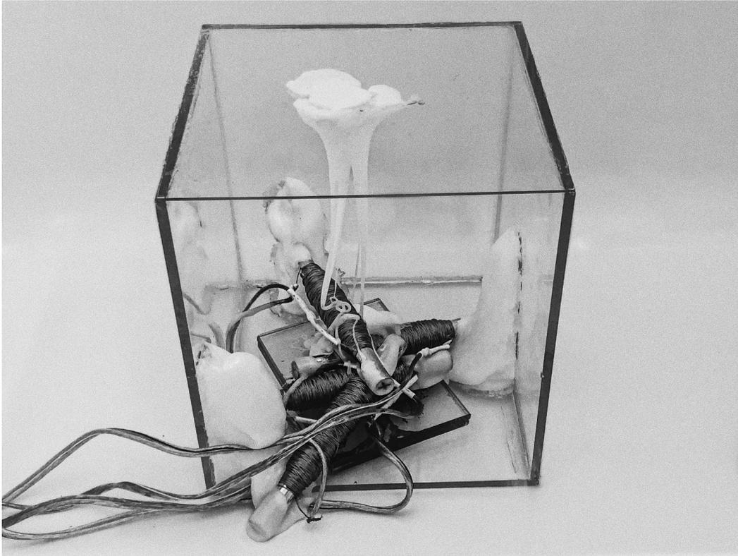
**Figure 46.** *The aftermath of my final recording session, when my electromagnet rig collapsed due to the plastic support melting.*
