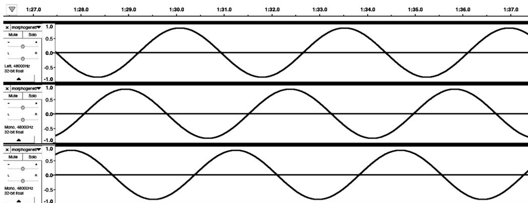
*Figure 44. These three-phase sine waves were amplified and sent through the three exterior coils, while the central coil was powered by a constant direct current.*
