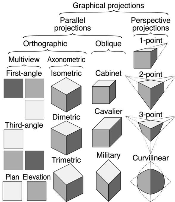
**Figure 10.** Diagram showing relationships between some types of 3D to 2D projections by CMG Lee from Wikimedia Commons
