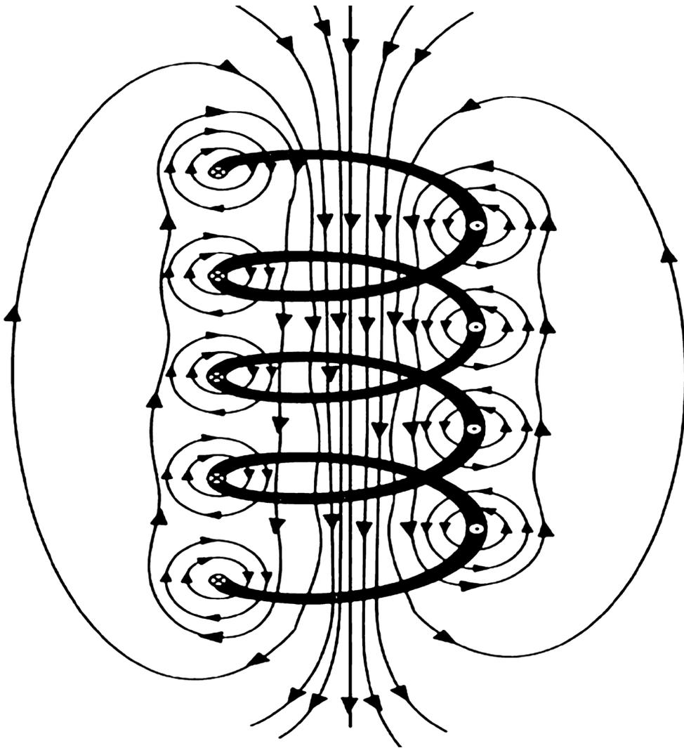
*Figure 22. A visualization of the magnetic field around an electromagnetic coil.*
